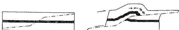
Fig. 19 - Schematic diagram to illustrate fold geometry resulting from shear strains within a thrust sheet moving above an irregular ramp-flat thrust surface (from RAMSAY, 1989).
