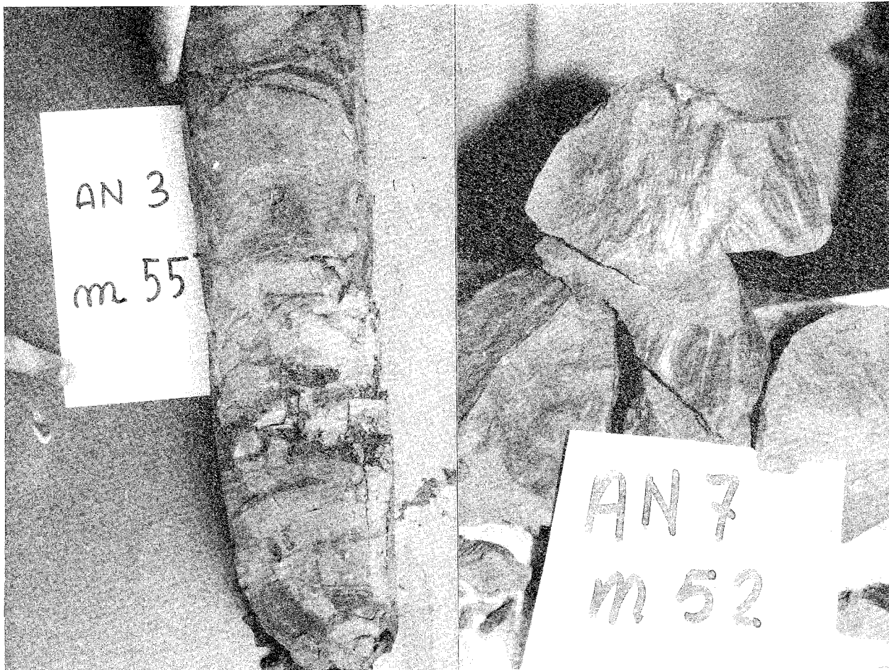
Fig. 7.5 - Livelli frantumati e liscati rinvenuti a 55 m ed a 52 m nei sondaggi AN 3 e AN 7. Broken and smoothed rock, sampled at the depth of 55 and 52 m in AN 3 and AN 7 boreholes.
